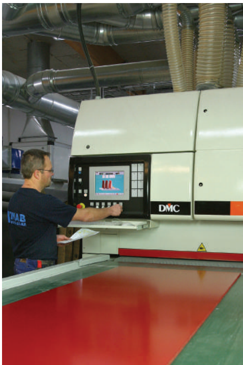
Computer controlled production line for surface treatment of wall units.
